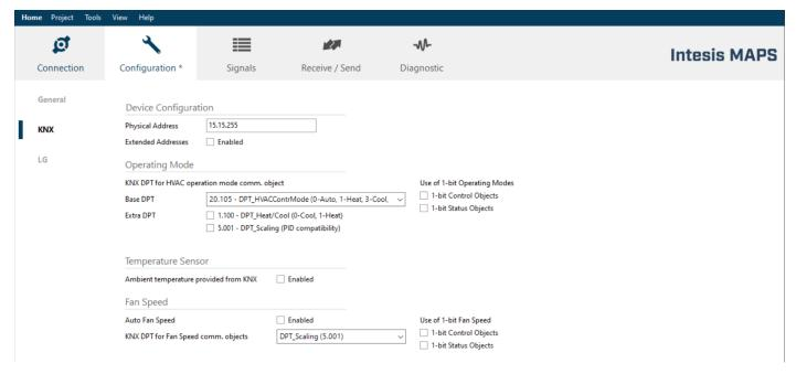
Figure 4.3 Intesis MAPS KNX configuration tab
