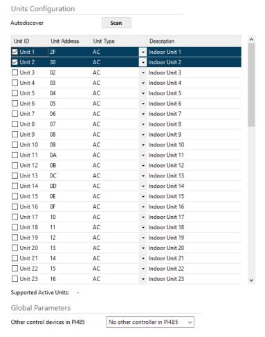
Figure 4.8 Intesis MAPS LG configuration tab after importing scan results
